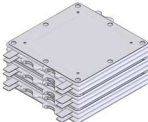
Figure 2 100 W fuel cell module based on the proposed design concept. Fuel, oxidant and cooling ports are at the side
