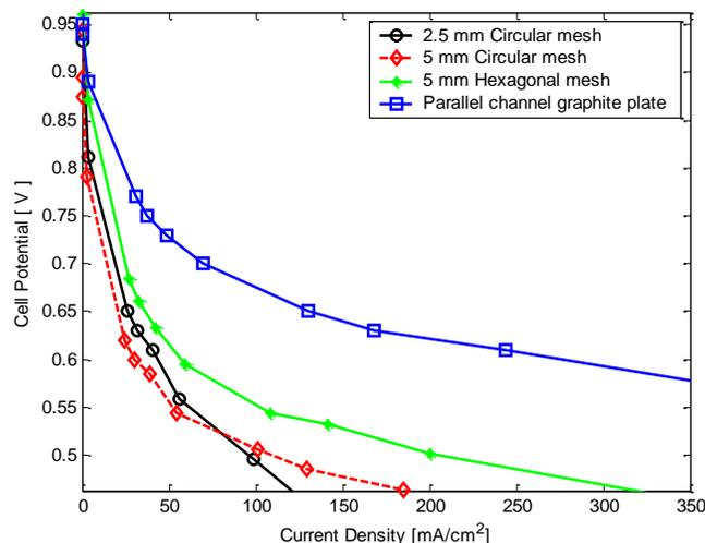
Figure 3 Test data for 3 meshed stainless steel electrode FCs and single conventional FC. Op. conditions 92% RH, 60°C
