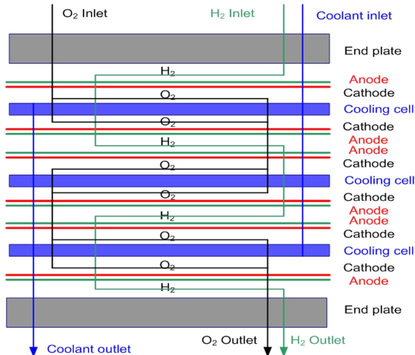
Figure 1 Schematic of FC design concept indicating gas flow and electrode arrangement
